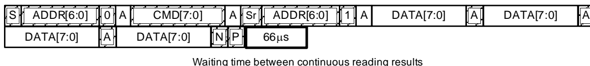
Figure 9. I 2 C Command Waiting Time
