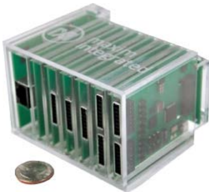
Figure 4. Maxim's Micro PLC Reference Design shows how much space can be saved when engineers take advantage of the latest advances in analog integration.
