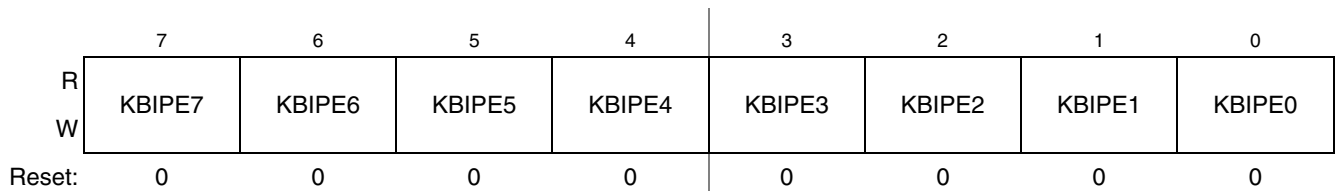
Figure 4-14. KBIx Interrupt Pin Select Register (KBIXPE)
