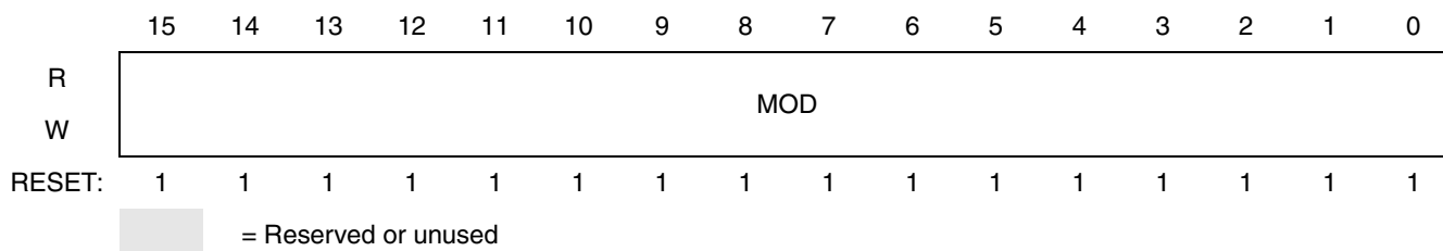
Figure 22-4. PDB Modulus Register (PDBMOD)
