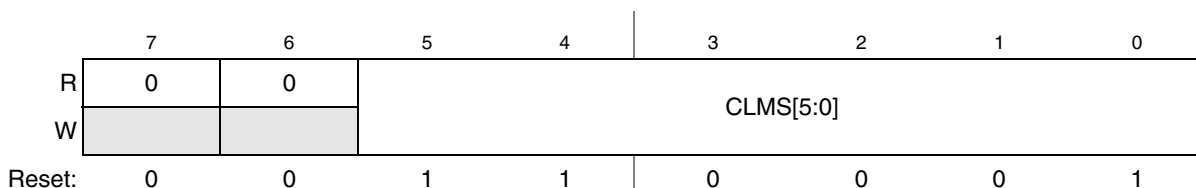
Figure 21-29. Minus-Side General Calibration Register (ADCCLMS)
