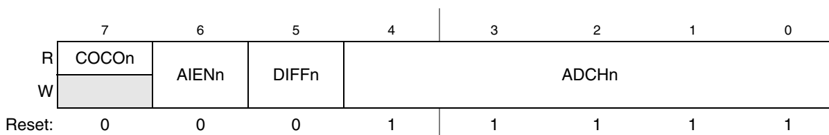
Figure 21-2. Status and Channel Control Register 1n (ADCSC1n)
