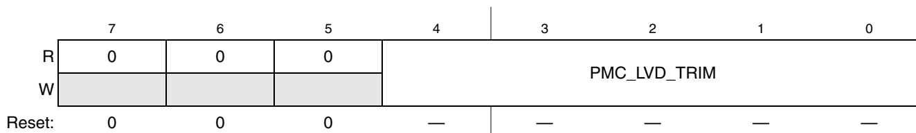
Figure 7-7. System Options 2 Register (SOPT2)
