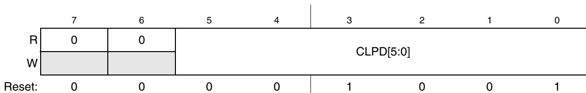
Figure 21-19. Plus-Side General Calibration Register (ADCCLPD)
