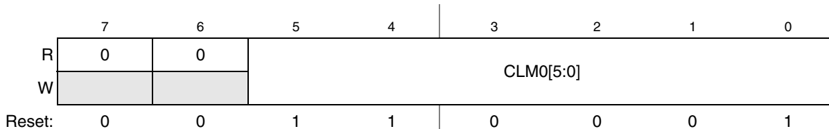
Figure 21-36. Minus-Side General Calibration Register (ADCCLM0)
