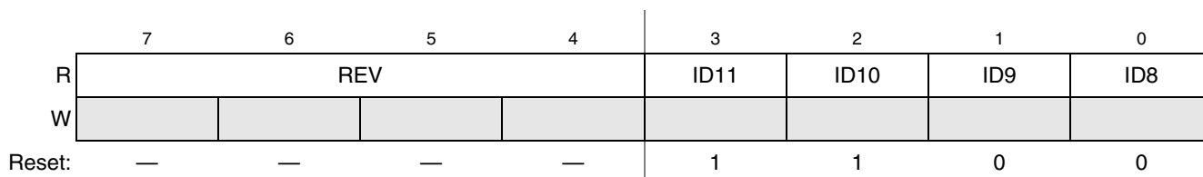
Figure 7-8. System Device Identification Register — High (SDIDH)
