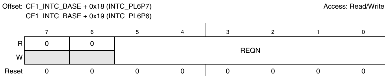
Figure 10-3. Programmable Level 6, Priority {7,6} Registers (INTC_PL6P{7,6})
