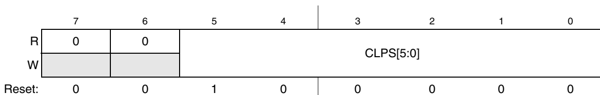
Figure 21-20. Plus-Side General Calibration Register (ADCCLPS)
