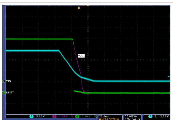
Figure 24. TPS7B6750-Q1 Power-Down Waveform
