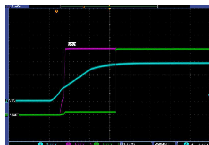
Figure 23. TPS7B6750-Q1 Power-Up Waveform
